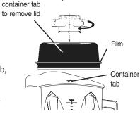
Figure A Always latch lid when processing hot liquids. See warning on page 3.
